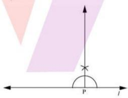
(ii) The compass is then adjusted up to the length of 4 cm. Construct an arc to intersect this perpendicular at point X. Considering any point Y on line l, join X to Y.
