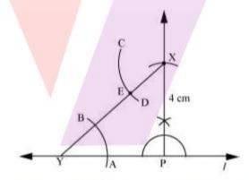
(v) The compass is adjusted up to the length of AB. Keeping the compass intact and taking E as the center, construct an arc to intersect the previously drawn arc CD at point F.
