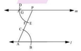
(vi) Join P to any point Q on line l. Consider another point R on line m. On similar grounds, a line can be drawn through point R and parallel to PQ.
