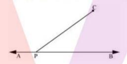
(ii) Taking P as center and with any convenient radius, draw an arc intersecting line AB at point D and line PC at point E.
