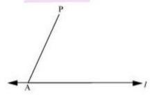
(ii) With A as center and with any convenient radius, draw an arc cutting l at B and AP at C.
