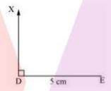
(iii) Since, DF measures 3 cm, with D as the center, cut an arc of radius 3 cm such that it intersects the ray DX. The point of intersection is the required point F.
