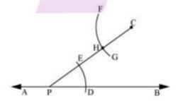
(iv) The compass is adjusted up to the length of DE. Keeping the compass intact and taking H as the center, draw an arc to intersect the previously drawn arc FG at point I.
