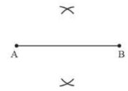
(iii) Let the points of intersection be C and D. Join them to obtain the perpendicular bisector of AB which cuts it at a point say M. Thus, M is the mid-point of AB.
