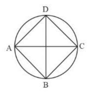
Upon joining the two diameters that are perpendicular to each other, we obtain a square.
