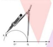
(f) Upon joining the points O' and R, we obtain an exact copy of the supplement angle of 40°.
